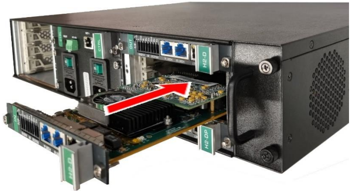
Figure 7: Input / Output Card Installation on the MTX3-16-M
